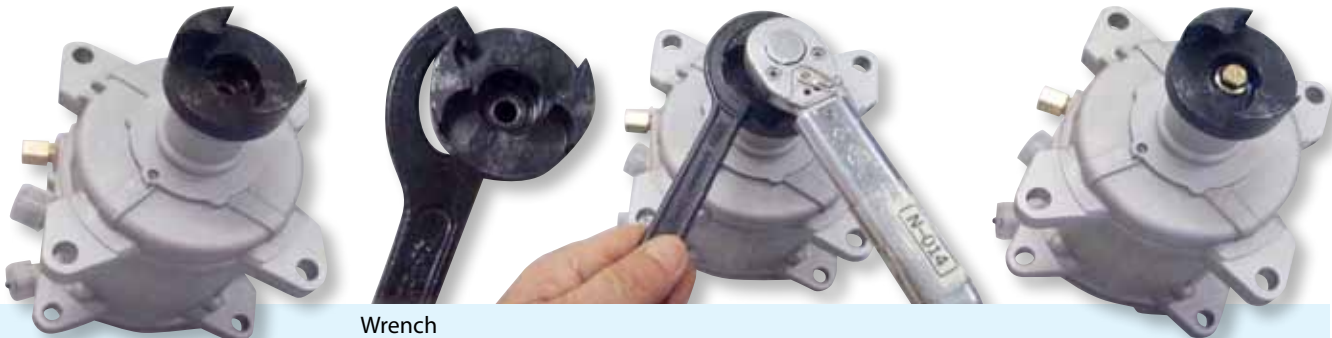
Insert coupling connector A into compressor
