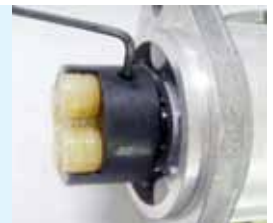
Fix coupling connector B and cushion to hydraulic drive motor shaft. Tighten with screw (M6)
