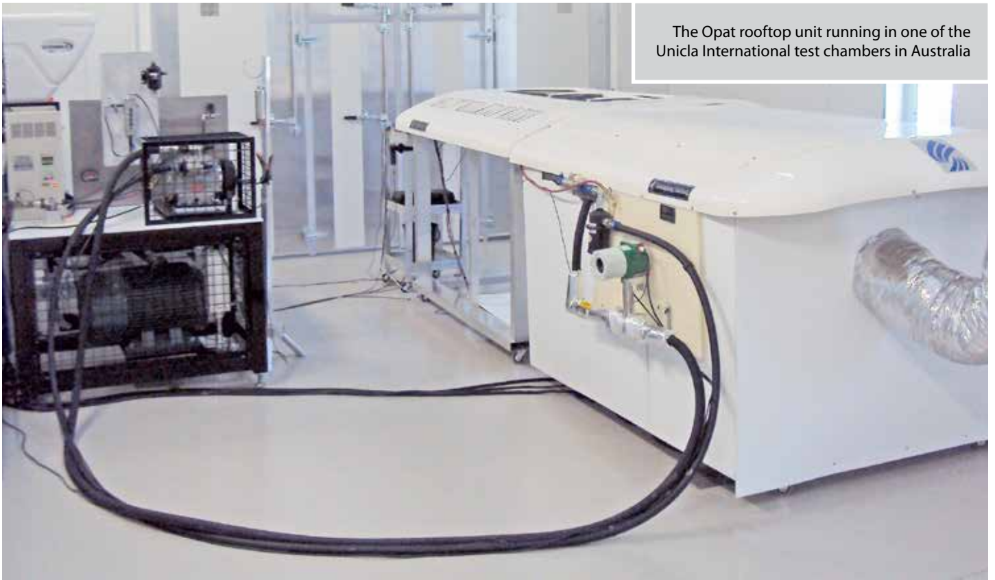
The Unicla UWX550 compressor connected up to the Opat rooftop unit
